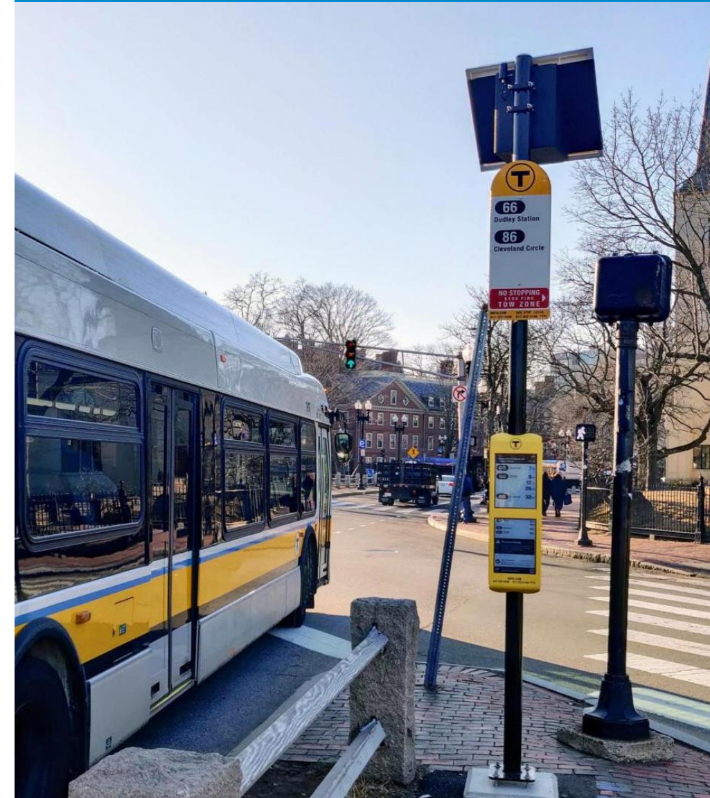
Solar e-paper display at MBTA bus stop
